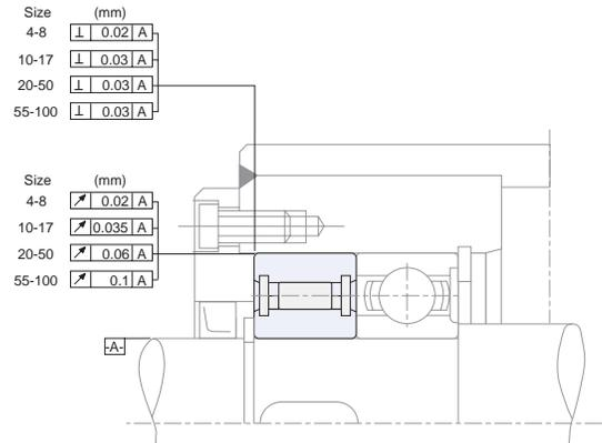
The AS clutch must be mounted adjacent to bearings to provide the concentricity and to support any axial and radial loads. Oil or grease lubrication must be provided along with seals to retain the lubricant.
